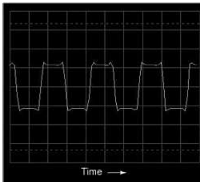
Figure 7.31: Oscilloscope time-domain display of a square wave
