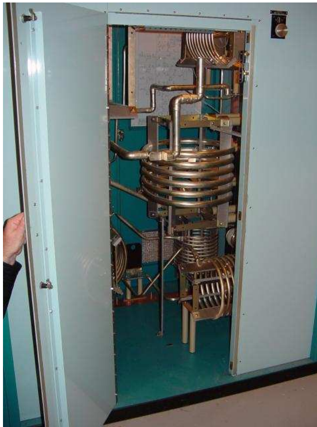
Figure 3.18: High power inductors formed from hollow tubes.
