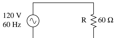
Figure 11.1: Ac source drives a purely resistive load.
