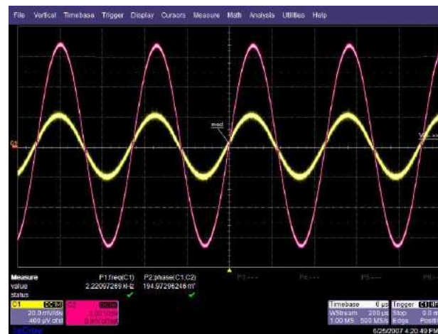
Figure 8.3: OPA227 A_v=50\text{dB} @ 2.2 kHz
