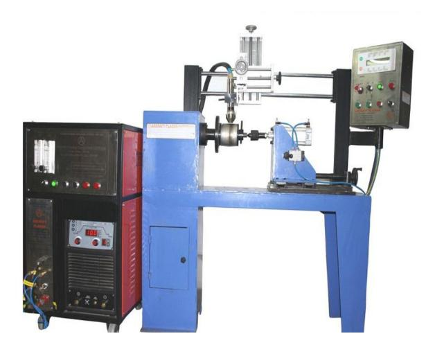
The **Arcraft Plasma Welding Lathe** has been innovatively engineered to provide a versatile platform for high production circumferential welding applications with superior accurate and repeatable results .
